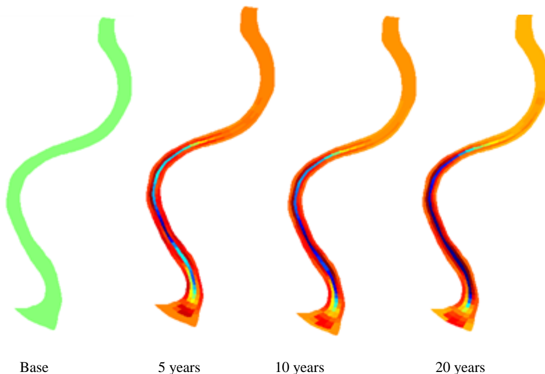
Figure 6.18: Simulated time series maps of erosion-sedimentation in the Kohelia River with the Delft 3D model (Note: The deep blue color indicates erosion, the deep red sedimentation and others indicate more or less no change).
